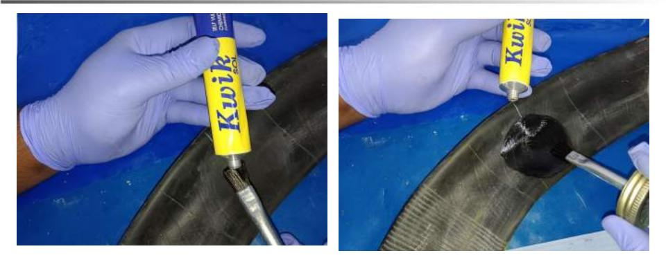
Apply a thin coat of Kwik Sol on the prepared area and let it dry. Ensure that there is no contamination on this coated area. Give about 5 minutes drying time.
