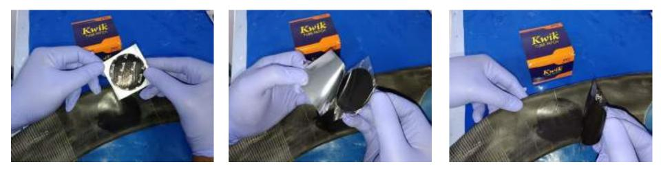
Remove the film from the Tube patch and make sure your fingers do not touch the exposed surface of the patch.
