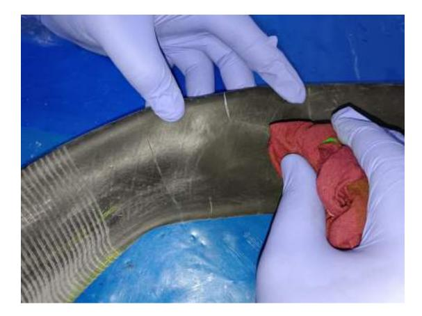
Clean the sanded area using a CLEAN DRY CLOTH. Ensure that oil or any other material like sand/water, does not contaminate the sanded area
