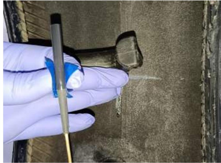
**Remove the Poly film from the Stem Plug patch. without touching the cushioned surface**
