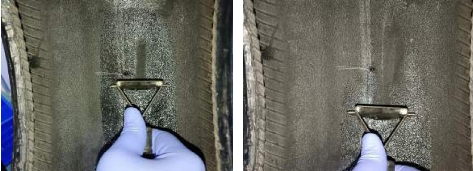
To clean, use Kwik Klean or any tire pre-buff cleaner or rubber solvents. While the area is still moist, use a tire scraper to remove all traces of dirt and silicone mold lubricant from the inner-liner area.
