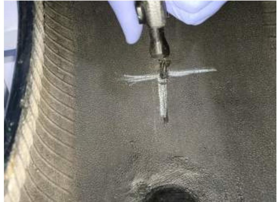
**Apply the Kwik Fast Dry Cement into the injury channel using a Spiral Cementing Tool**
