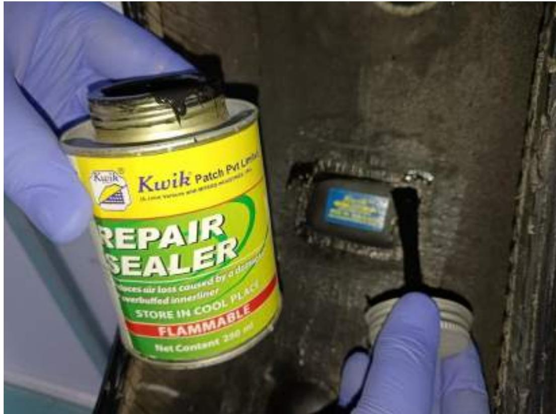
**Apply a coat of Kwik Repair Sealer around the patch and entire exposed buffed area.**
