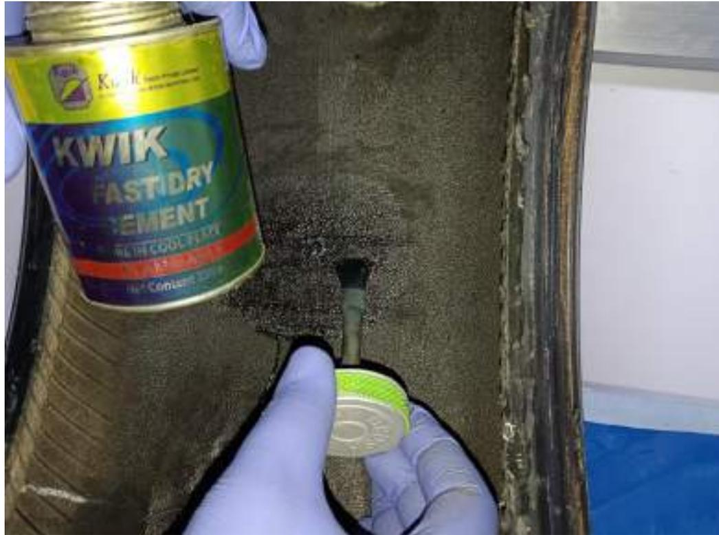
**Apply a Single Coat of Fast Dry Cement in a stippling motion and allow it to dry (Normal drying time is 3 to 5 min. or as per the ambient temperature and humidity).**
