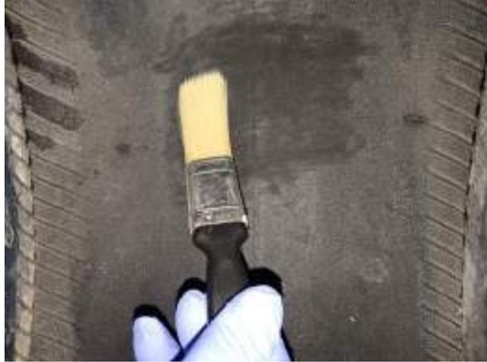
**After rasping the area, clean the buffed dust with a nylon brush or vacuum the dust thoroughly.**
