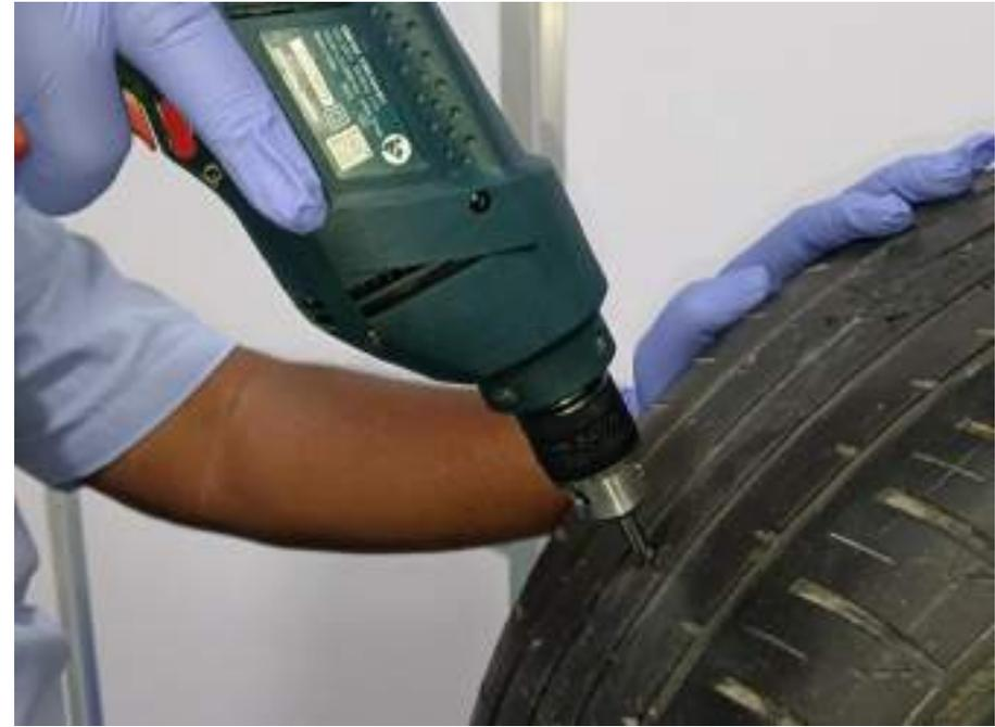
**Use a Low Speed Drill (max 1200 rpm) and an appropriate size carbide cutter to prepare the injury.**
