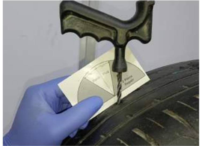
**Remove the foreign material from the injury and using a probe or an inspection tool, determine the size and angle of the injury.**
